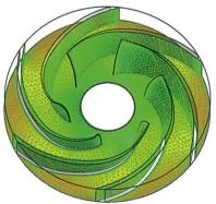
CFD designed impellers and diffusers to optimize the hydraulic performance.
